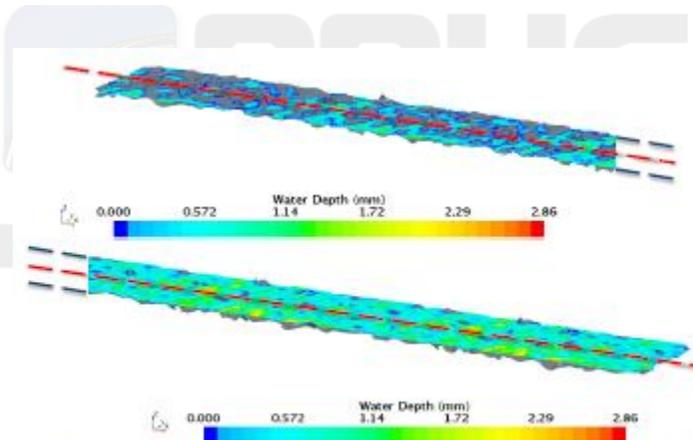
Figure 5-3: Water depth on a rough pavement, (a) close to the median, (b) close to the shoulder. Rainfall intensity 2 in/hr, slope 2%.
