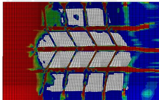
Volume fraction of the water flowing in the tire pattern groove with 5-mm WFT at 40 mph.
