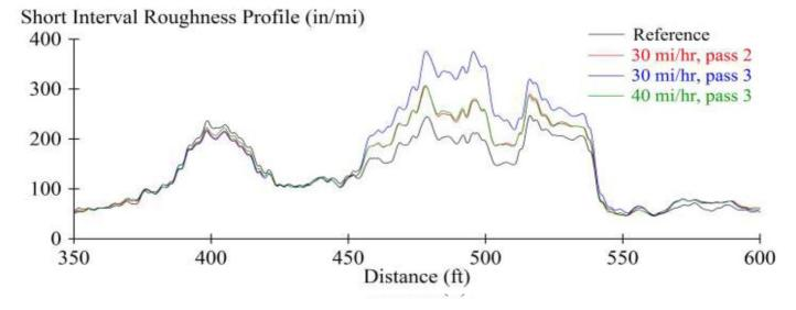
*Figure 34. Roughness profiles of transversely inconsistent localized roughness.*
