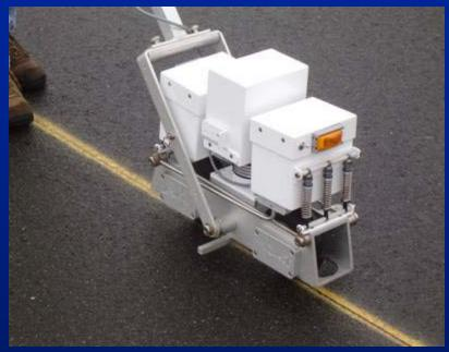
Able to obtain data at 1-inch interval at walking speeds
