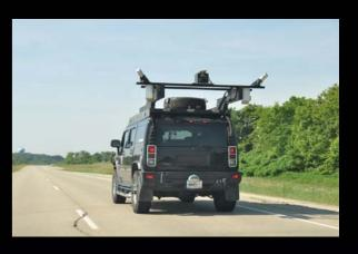
Transverse crack detection:
